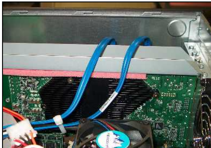
HP Workstation xw6000 cable routing (shown with AGP support bracket)
